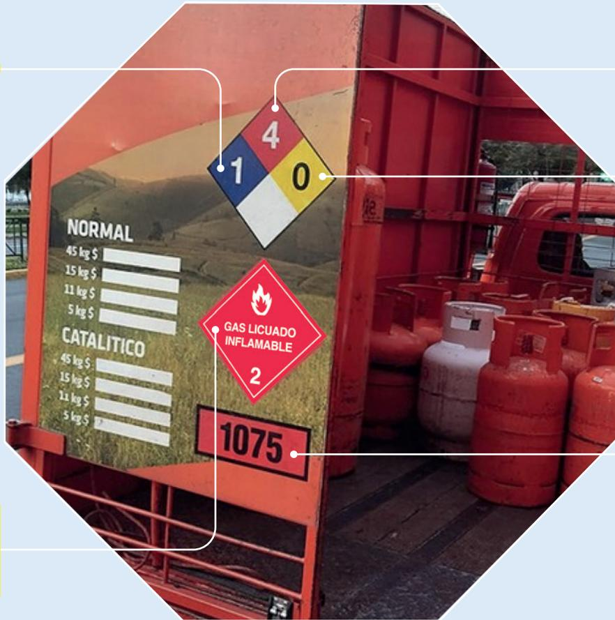
The diagram shows the rear of a red gas truck. On the side panel, there are two hazard labels: a diamond-shaped label with the number '1075' and a red diamond label with a flame icon and the text 'GAS LICUADO INFLAMABLE' and the number '2'. Below these labels is a black rectangular label with the number '1075' in white. To the left of the labels is a list of weights for 'NORMAL' and 'CATALITICO' gas cylinders. The truck is loaded with several red and white gas cylinders.
